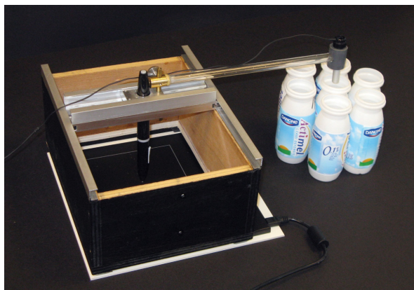
Fig. 2. A two-dimensional acoustic scanning device that collects data for computer visualization.
